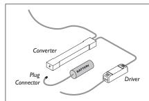
For Emergency versions ensure the battery plug connections are made prior to a permanent mains supply being present and this is maintained for a minimum 24hrs to ensure correct operation.
