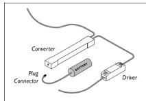
For Emergency versions ensure the battery plug connections are made prior to a permanent mains supply being present and this is maintained for a minimum 24hrs to ensure correct operation.
