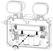
Reconnect the electrical supply and test the installation.
