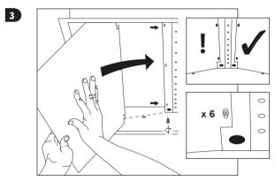
When sliding reflector in, do not slide over LED's
