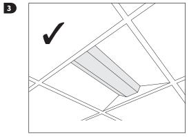
Insulation etc. should not cover body or remote gear
