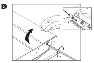
For Emergency versions ensure battery bullet connection is made only when a permanent mains supply is present
