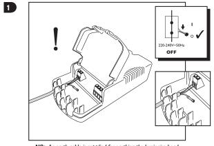
**NB:** An earth cable is supplied for earthing the luminaire head
