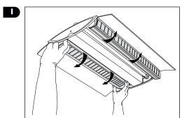
NB - Squeeze vertical face of refractor to disengage from screw and allow to pivot down.
