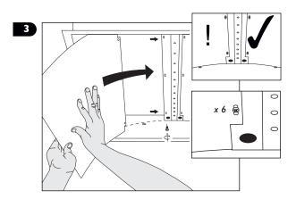
N.B. - When sliding reflector in, do not slide over LEDs
