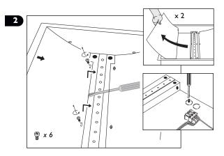
N.B. - When sliding reflector out, do not slide over LEDs
